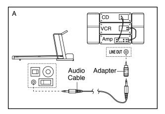
B. Plug one end of the audio cable into the jack on the front of the treadmill near the power cord. Plug the other end of the cable into the included adapter. Plug the adapter into an RCA Y-adapter (available at electronics stores). Next, remove the wire that is currently plugged into the LINE OUT jack on your stereo and plug the wire into the unused side of the RCA Y-adapter. Plug the RCA Y-adapter into the LINE OUT jack on your stereo.
